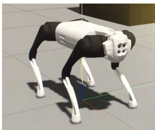
Figure 22: Unitree Go1 robot achieving successful stand-up using open-loop control.
