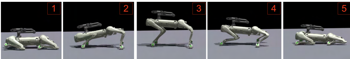
Figure 48: Isaac Gym simulation: stand-up policy and open-loop seating.
