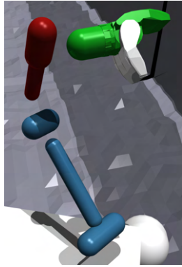
Figure 21: Collision meshes of the arm (link 02 in blue, 03 in red and 06 in green).
