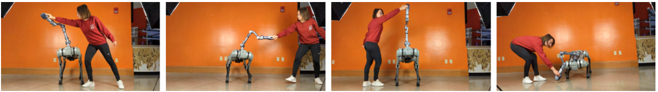
Figure 69: Robot in compliant mode, with coordinated posture ensuring the gripper’s steady position.
